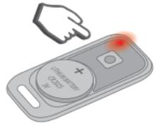
4) Successful registration will be confirmed by a green flash SMS message. If the tag is not registered, the LED will light up red.
