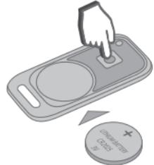
3) Release the button and check presence of a red flashes series for 10 seconds.
