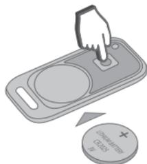
3) Release the button and check for a series of red flashes within 10 seconds.
