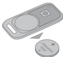
2) Push and hold the tag button and insert the battery inside again. The LED will turn to red.
