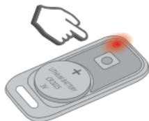
4) Successful registration will be confirmed by a green flash and a response SMS. If the tag is not registered, the LED will turn red.
